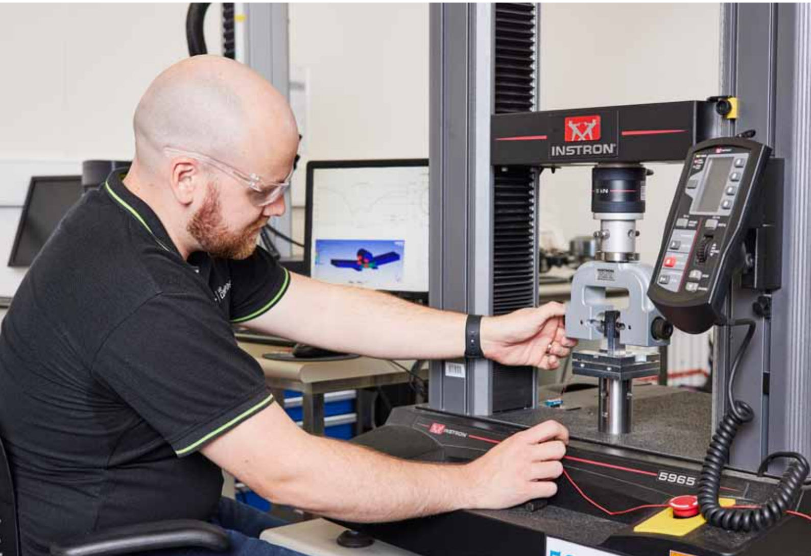
Dr Mitch Dunn from UQ tests the strength of the coaxial radio-frequency connector of a functional antenna structure. The DMTC project team is investigating the electromechanical performance of different connector attachment options to optimise the durability of these critical system components. More information on the project is on Page 32.
