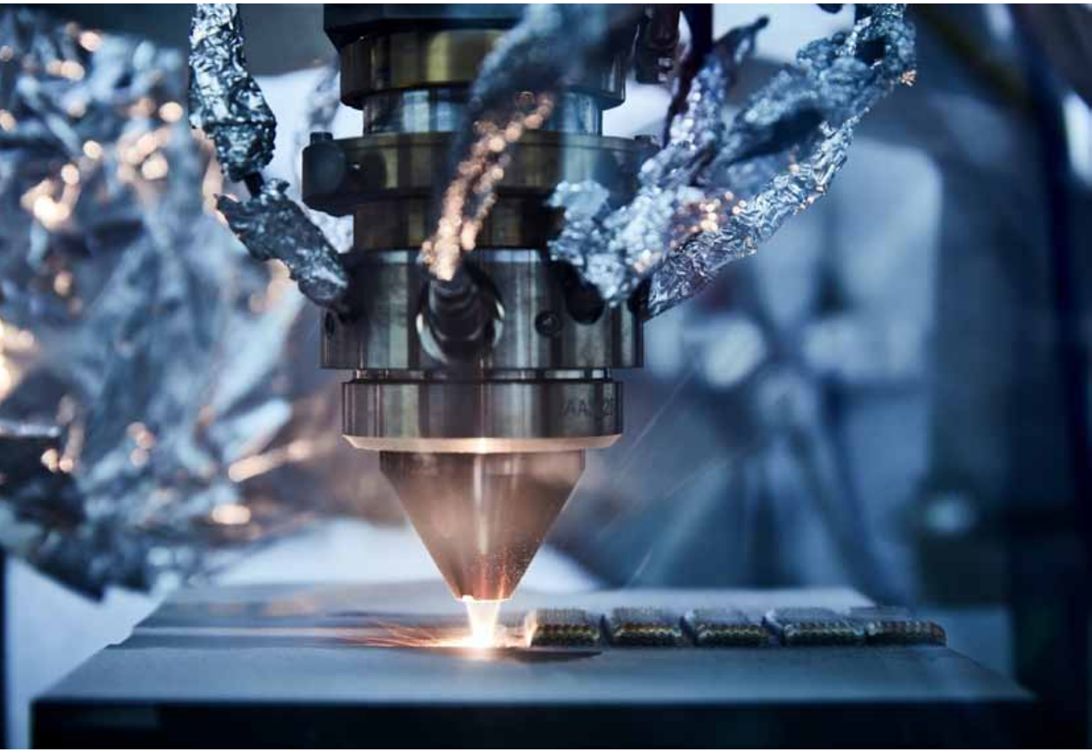
RUAG Australia is working with DMTC's Air Program and research partners to advance the development and application of laser additive deposition (LAD), a highly efficient repair process for aerospace components that offers significant cost and lead-time advantages over the need to replace the part.
