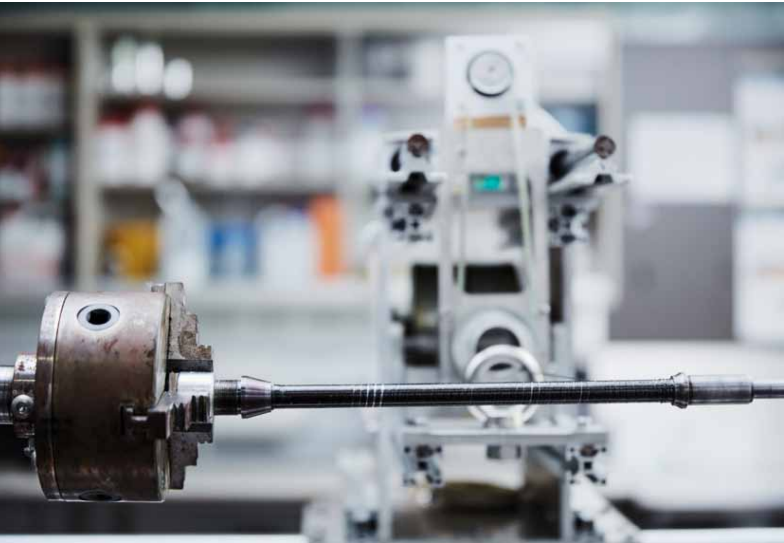
Lightweighting for next-generation small arms: carbon filament passes through a resin bath and is wound in a pattern best suited to the intended loading directions of the component.
