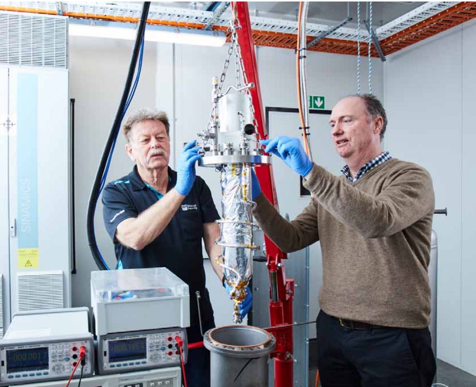
L to R: Along with their team, Queensland University of Technology's (QUT) Mr Robert Hickey, Senior Technician, and Mr Peter O'Brien, Research Fellow, testing cryocooler equipment to ascertain whether the benefits of high temperature superconductors can be harnessed by naval fleets.
