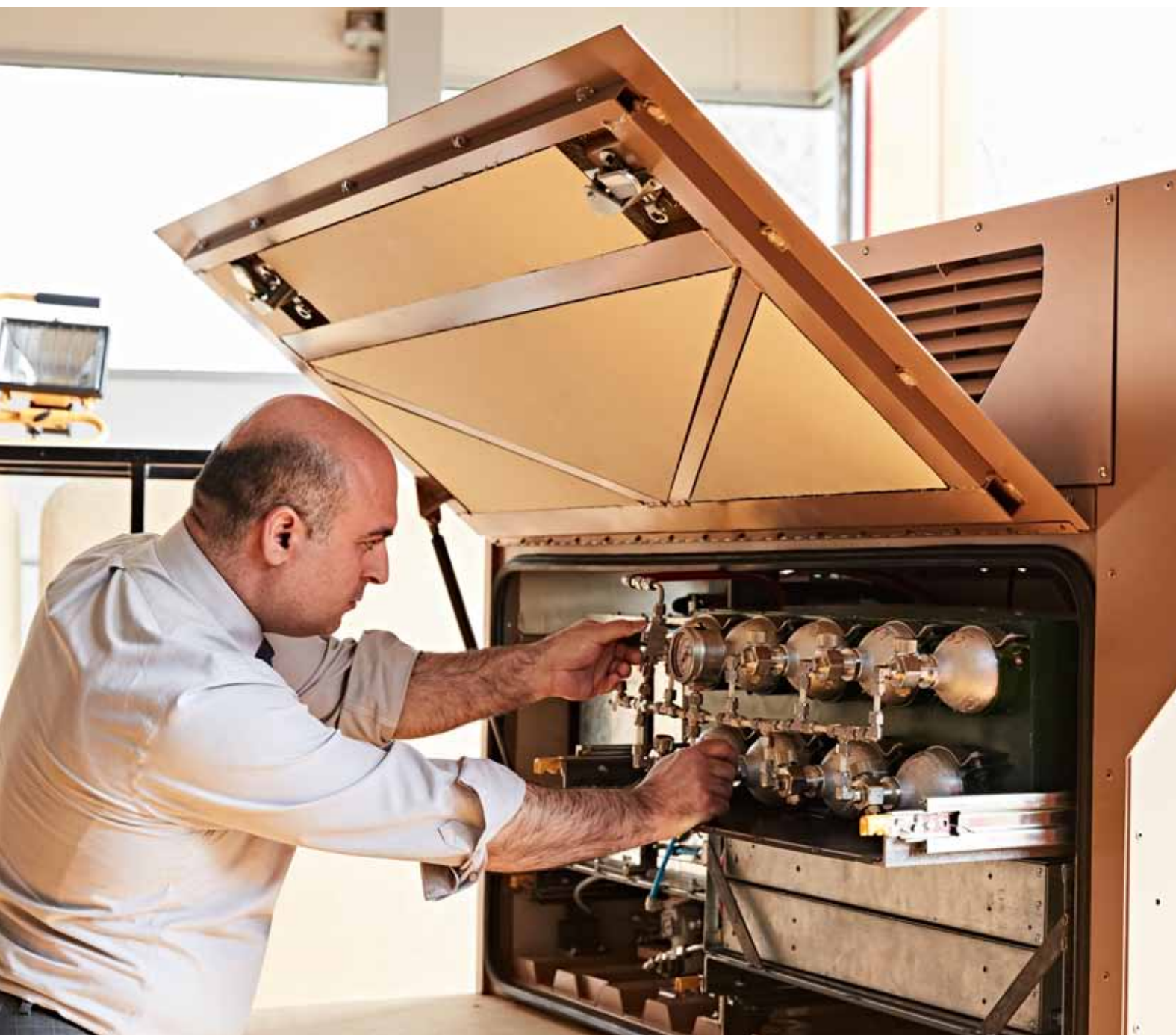
Dr Bahman Shabani, Senior Lecturer at RMIT Bundoora checks the hydrogen fuel cell, which has a maximum capacity of 5kW. The electronic load bank draws power from the fuel cell to demonstrate the load and can be varied to simulate different uses of the power by auxiliary functions.
