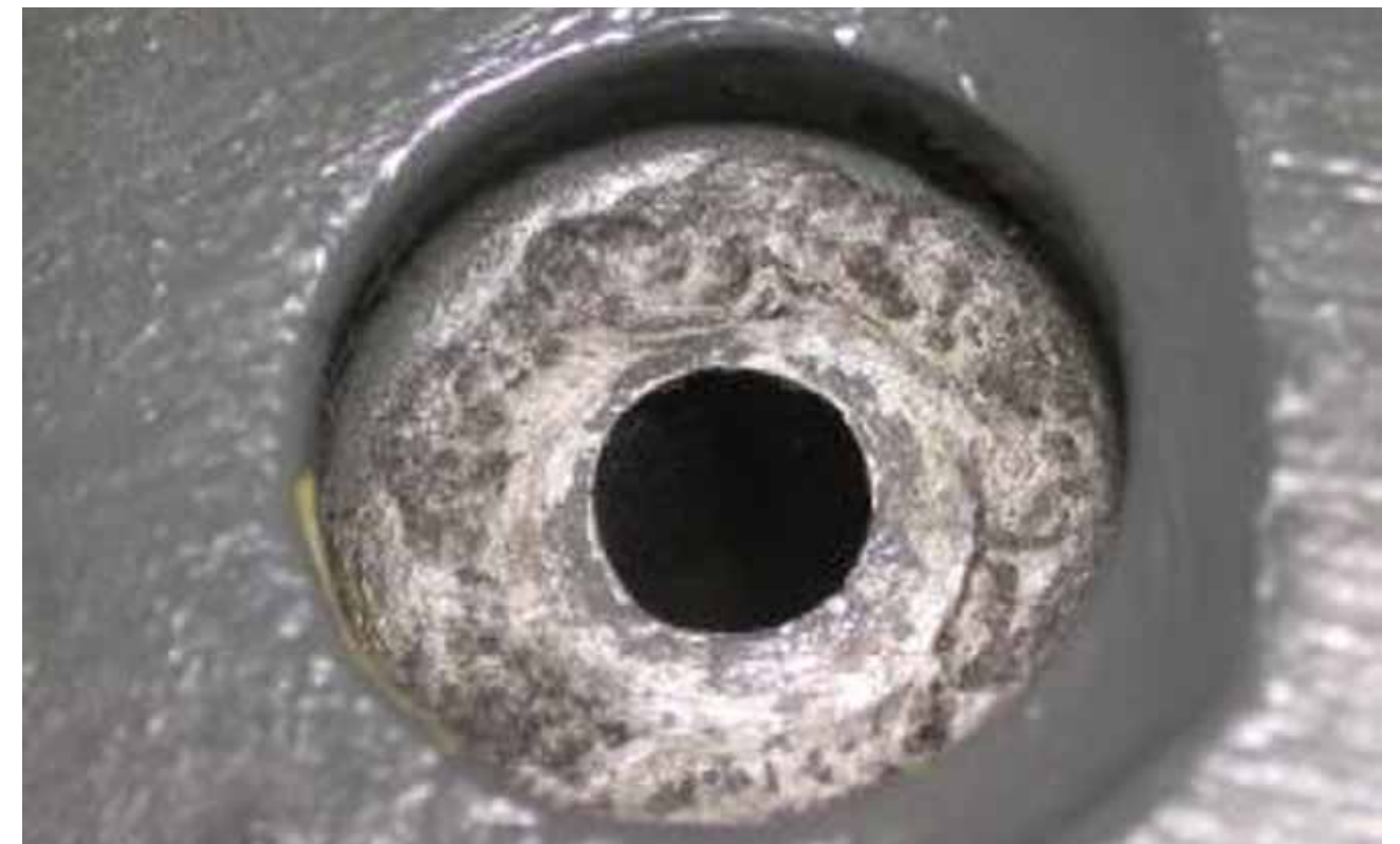
Legacy magnesium alloys including the ZE41A-T5 compound used on gearbox housing components are noted for their strength and hardness but suffer from poor corrosion resistance.
